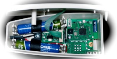
View of Cluster Node Board
